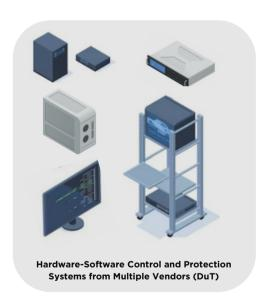
Dynamic performance of a wide range of embedded control and protection components (i.e. DuT), are verified. Wide range of electric grid signals such as voltage, current and breaker status are sent to the DuT
